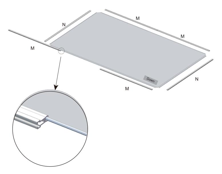
4. Center the inner frame on the back of the screen surface.
