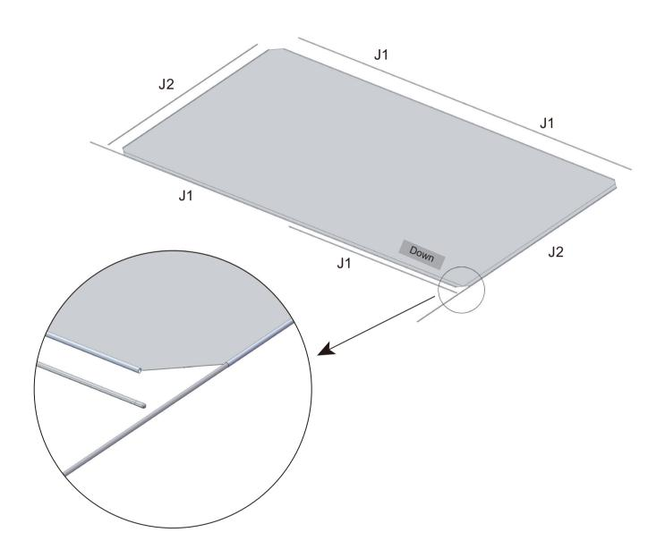
3. Slide the screen edges into grooves of the pull rod (N) and pull rod (M) as shown in the illustration below.
