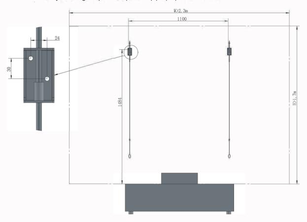
2. Tear off the protective films on the four corners of the screen. The screen stands upright, and the **Down** label on the back of the screen is at the bottom. After the screen is hung on the wall, rotate the adjusting rod to adjust the height of the screen to achieve the best display effect.
